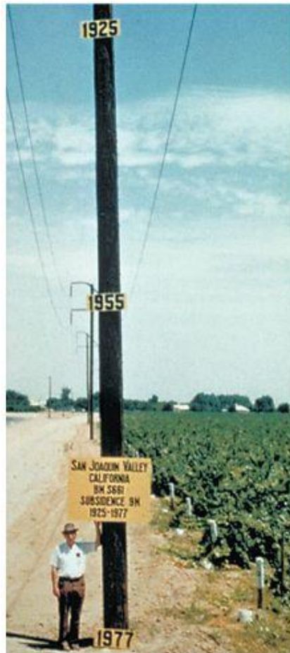
Figure 6: Excessive use of groundwater over time has led to groundwater basin depletion and substantial subsidence of land. This 1977 photo shows how many feet the land subsided as a result of groundwater withdrawal in the San Joaquin Valley from 1925 to 1977. (Photo: USGS, 1977)
