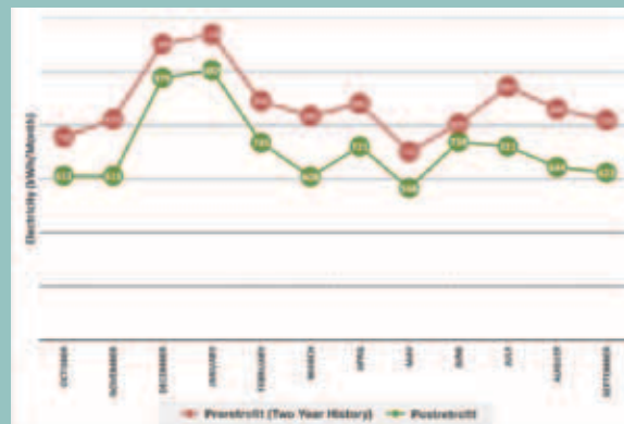
Figure 1. The Stockings' electricity use before and after retrofit.
