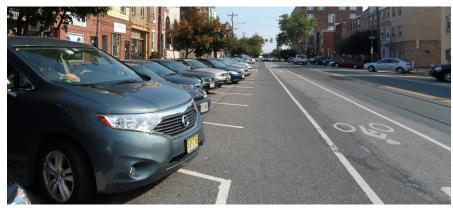
FIGURE 20: BACK-IN ANGLED PARKING IN COMBINATION WITH A BIKE LANE
