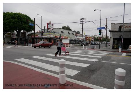
FIGURE 9: IMAGE OF TEMPORARY CURB EXTENSIONS WITH LOW-COST MATERIALS
